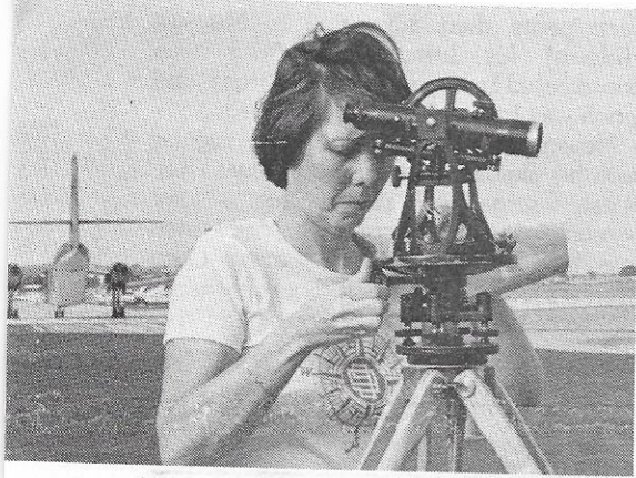
Gloria Burlette setting up the transit to line up our points on the New Orleans 99 compass rose.
